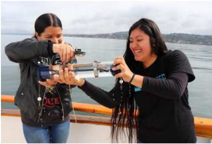
Students use a Van Doren sampler during a floating lab. Photo by WILDCOAST
